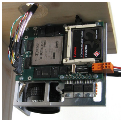
Fig. 1 On-board image processing system for small UAVs; foreground: image processing unit; background: aluminum frame, downward facing camera lens; backside (not visible): camera, power supply, CAROLO on-board navigation computer.
