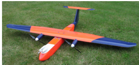
Fig. 2 CAROLO T200 (pictured here with wind measuring 9-hole-probe and other meteorological sensors).
