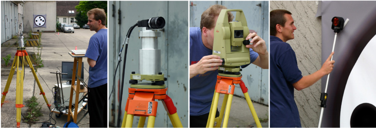
Fig. 7 Experimental installation, camera on adapter, geodesy tachymeter, measuring the marker corner points.
